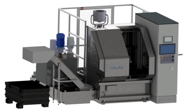
The universal two-axis lathe with horizontal main spindle has been built to reduce space requirements while maintaining high performance. The turret (optionally with driven tools) is static, while the spindle is on a cross slide. The machine can be equipped with hydraulic clamping, high-pressure water cooling or a probe. This compact lathe features a wide range of available options to customize your machine to your exact needs, including workpiece loading and unloading automation.
